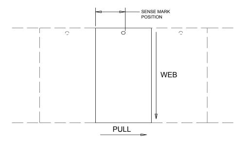
If it is a hole sense mark the command is  $\sim$ XMH. If it is a reflective sense mark the command is  $\sim$ XMR. This command is followed immediately by the sense mark's position. If the 3" X 2-1/4" tag described above had a hole sense mark in the middle of the tag, the sense mark command would be  $\sim$ XMH1125. If the sense to cut distance is 0, a properly adjusted printer will cut at the leading edge of the sense mark.
