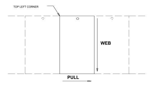
The point of reference to a field is also the top left hand corner. When a field of text is in a normal reading position so that the text can be read from left to right, the top left hand corner is the corner formed by the left edge of the first letter and the top edge of the letters. This is the point of a field that is used to position a field on a tag and also is the pivot point for a field when it is rotated.
