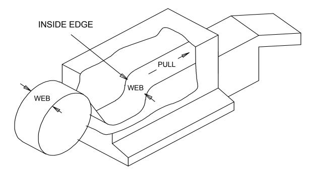
The pull and web directions are very important when laying out a tag / label. If these dimensions are not determined correctly then the orientations of the fields that are placed on the tag/label will be incorrect.
