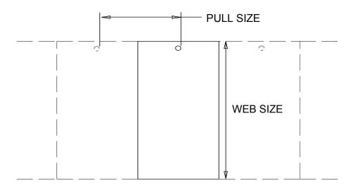
For a tag that has a web size of 3" the command would be  $\sim$ XW3000. (All measurements are in units of thousandths of an inch.) For a pull size of 2-1/4", the command would be  $\sim$ XP2250. If the tag is a sense mark tag, the best way to determine the pull size is to measure from the leading edge of one sense mark to the leading edge of the next sense mark on a continuous roll of stock.
